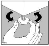
Level the washing machine by raising or lowering the feet. The feet may be tight to adjust as they incorporate a self locking nut, but the machine MUST be level.
